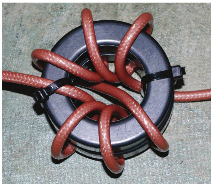
PHOTO 1: A 7-turn broadband common-mode choke.
