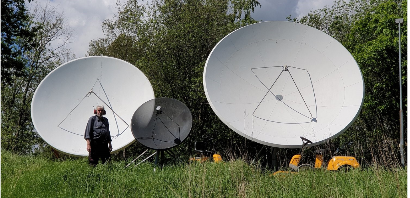
The 4.5m and 3.7-metre reflectors are for “Freesat” and the little black 1.3m is for the up/down link to QO-100 satellite.
