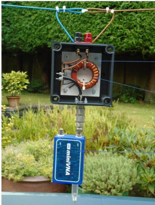
Photo. No 3 Testing 15m band trapped Dipole with 1:1 Voltage Balun
