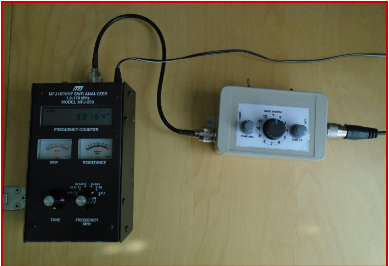
ABOVE: New Internal Layout No2 BELOW: Checking Performance with MFJ-259 Antenna Analyser
